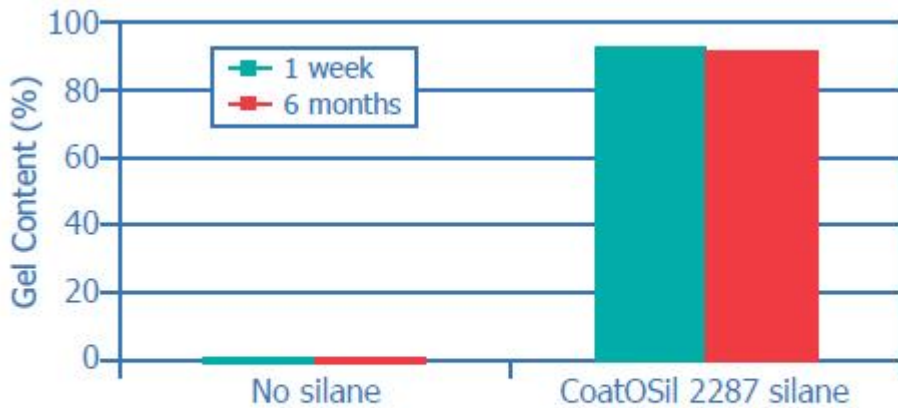
Figure 3: Gel Content of Acrylic Latex Coating Cured with CoatOSil 2287 Silane
