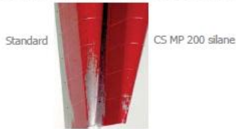
Ratio epoxy / amine 1 / 1 to 1.2 CoatOSil MP 200 silane 0 and 2% With or without 0.5% Catalyst
