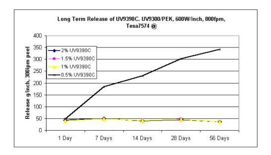
In the application illustrated in Figure 2, the film laminate liner permits use of 1 - 2 parts UV9390C in UV9300 without much effect on long term release stability versus the TESA test tape, but <1 phr catalyst may be insufficient.
